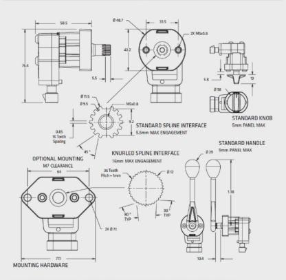
STANDARD MOUNTING: M5 X 0.8 X 30 PAN HEAD SCREWS RECOMMENDED. OPTIONAL MOUNTING: M7 X 1 X 30 PAN HEAD SCREWS WITH NUTS RECOMMENDED.
